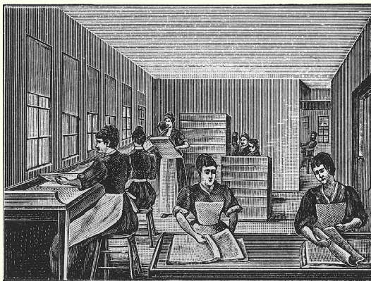
Fig. 20. Finally the paper is sorted into different quality levels and packed for shipment.
