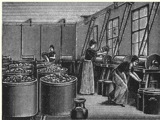
Fig. 16. The albumen is beaten to a foam using steam-driven churns.
